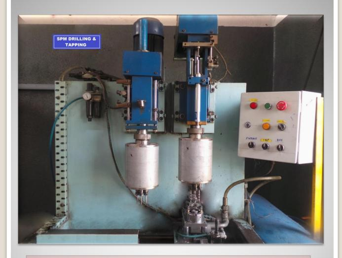
Machine Name - SPM. DRILLING & TAPPING
